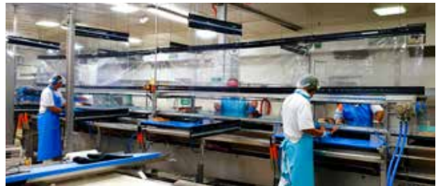
PVC screens were installed to maintain distance and keep Sealord factory workers safe during alert levels 1 and 2.
